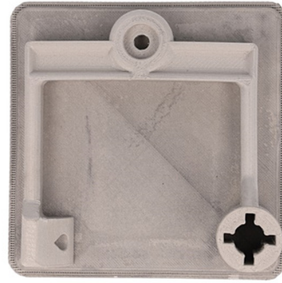
Figure 22. Use of shrinkage plate ensure uniform shrinkage
