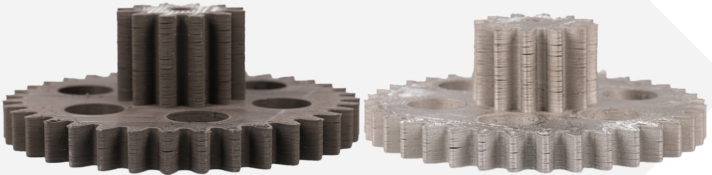
Figure 20. Print Delamination become sintered cracks
