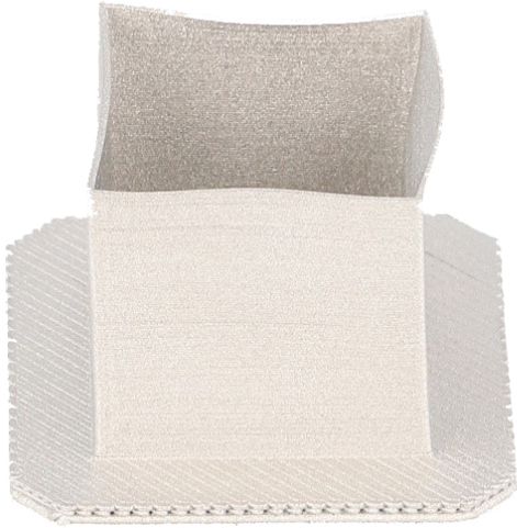
Figure 12. 0,4 mm Wall Failure
